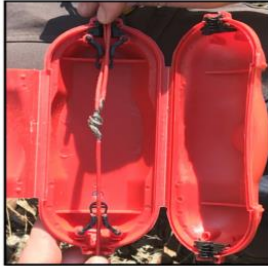
"Pill Box" enclosure Original engineered guarding control for electrode live conductors.
